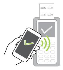
To do contactless payment or read data, you must turn NFC on. Make sure the NFC area (shaded) on the back of HTC Desire 20 pro is close to the terminal, card, or device when you tap your phone.
